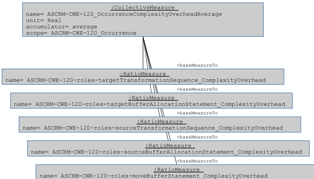
Figure 14: ASCRM-CWE-120 occurrence complexity overhead average with SMM CollectiveMeasure and RatioMeasures
