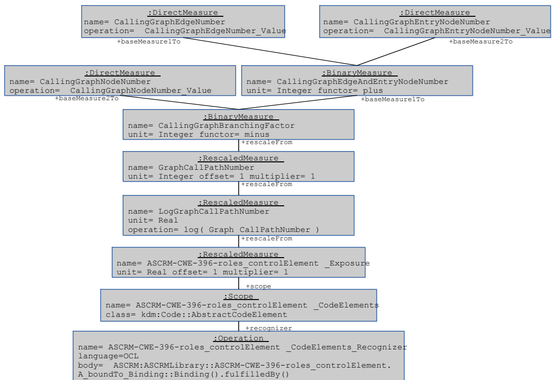
Figure 11: ASCRM-CWE-396-roles-controlElement role direct exposure computation with SMM OCLOperations, Operation, DirectMeasure, Scope, and Recognizer
