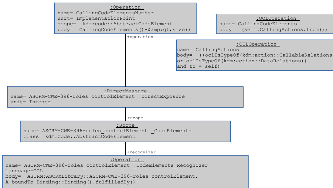
Figure 10: ASCRM-CWE-396-roles-controlElement role direct exposure computation with SMM OCLOperations, Operation, DirectMeasure, Scope, and Recognizer
