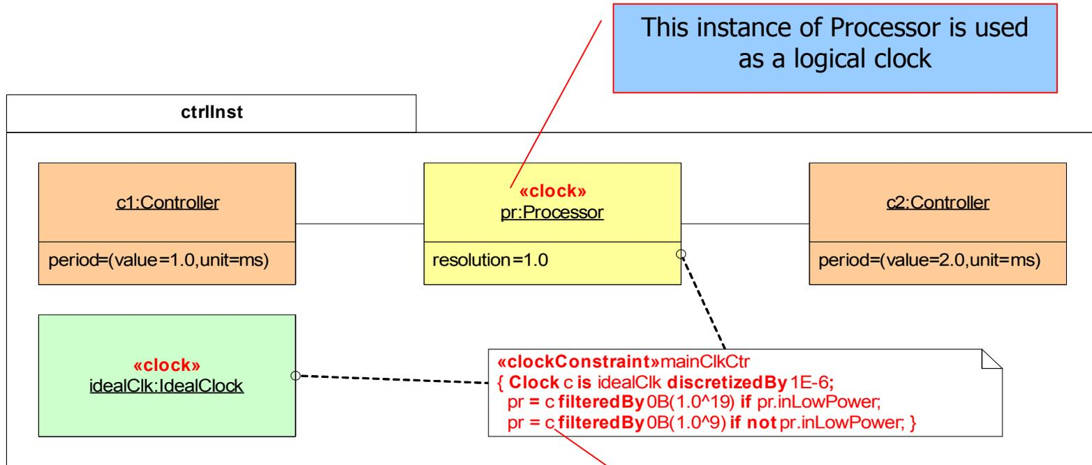
This instance of Processor is used as a logical clock
