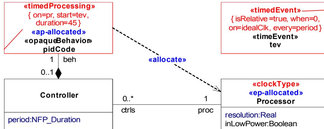
The pid code is triggered by tev and takes 45 cycles of Processor
