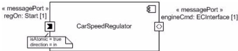
Figure 12.17 - Example of UML component with specialized MARTE ports
