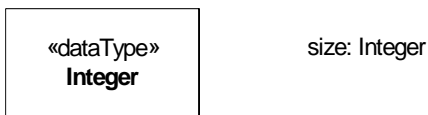
Figure 11.19 - Notation of data type: to the left is an icon denoting a data type and to the right is a reference to a data type that is used in an attribute.
