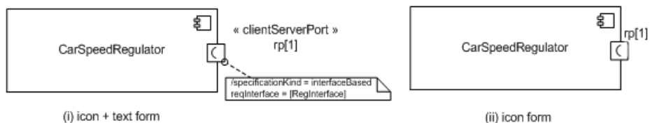
Figure 12.16 - Example of interface-based ClientServerPorts
